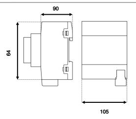
All values given in the device dimensions are in milimeters. The device can be used in an area with 6 modules.
